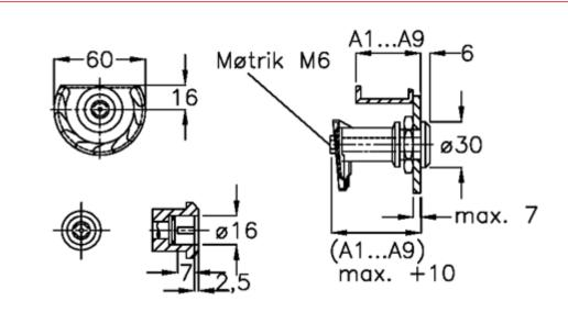
Door + frame thickness = 27-35 Measure type = A3
